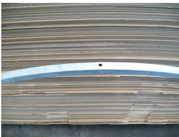
Identify the hole of the top of the arch and drill the cover by transparence (diameter 10 mm)
