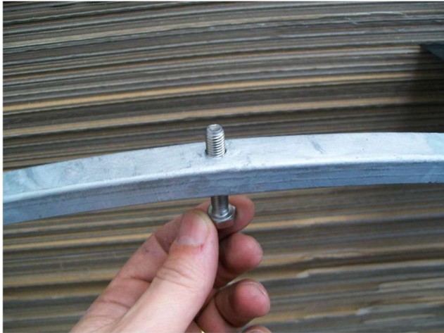
Put the screw M6 x 45
