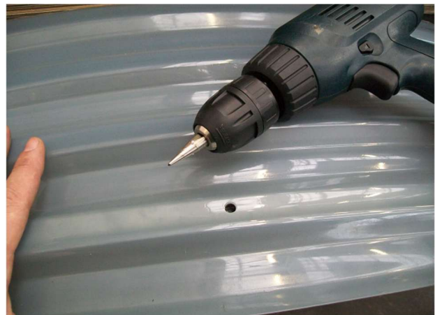
Identify the hole of the top of the arch and drill the cover by transparence (diameter 10 mm)
